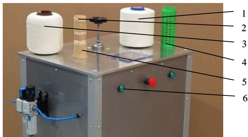
Fig. 2. Prototype of new package testing device based on the measurement of flow resistance. Two kinds of tested packages and plastic spring tube are also shown
