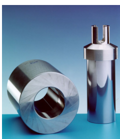
Fig. 8. Manufactured resonator for the NPL Boltzmann experiment [17].
