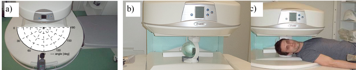
Fig. 1. An arrangement of noise SPL measurement (a) and noise recording in the MRI Opera using the testing water phantom (b), and a lying examined person (c).
