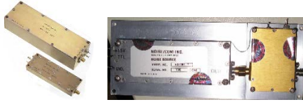
Fig. 3. The noise generator and power amplifier. The image shows the tested noise generator, whose output power is 0dBm in the frequency range of between 100kHz and 10GHz.
