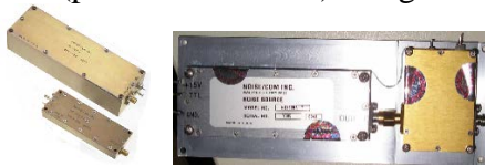
Fig. 3. The noise generator and power amplifier. The image shows the tested noise generator, whose output power is 0dBm in the frequency range of between 100kHz and 10GHz.
