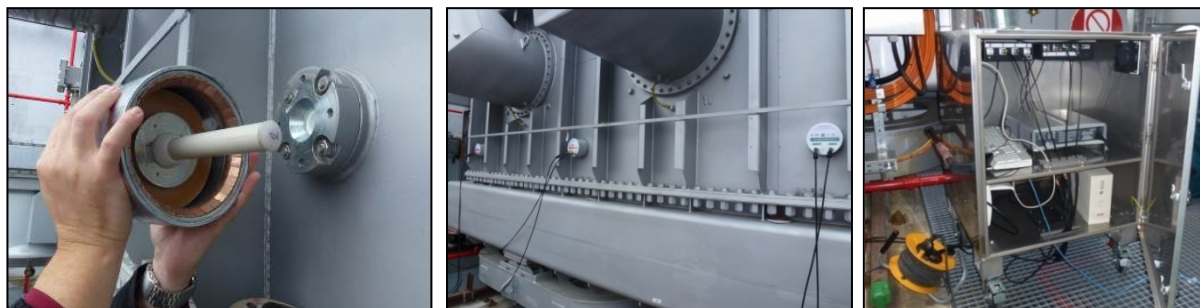
Fig. 1. Left - sensing head, middle - sensing heads mounted on the transformer, right – assembly of the diagnostic system in shielded box.
