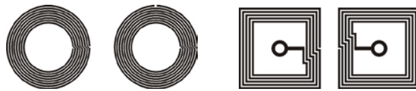
Fig. 5. Variations of the resonators with distributed capacitance.
