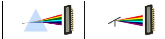
Fig. 04. Spectral sensor with prism (left) and grating (right)
