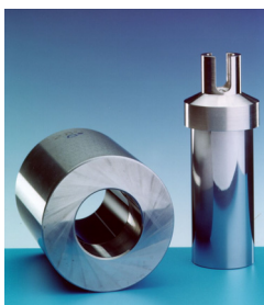
Fig. 8. Manufactured resonator for the NPL Boltzmann experiment [17].
